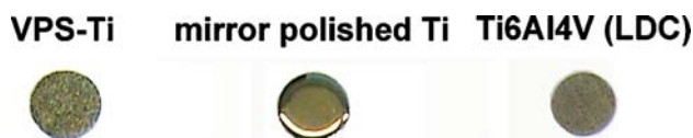
Fig. 1 Examples of the samples used in this paper. Since the mirror polished pure Titanium and Ti6Al7Nb samples optically look the same only one representative disc is shown
